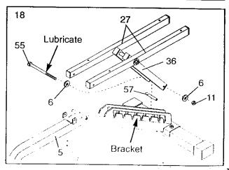
19. Lubricate an M1U.X.18Umm Boit (22). Attach the Backrest Tubes (27) to the Indicated Tube on the Bench Frame (5) with the Bolt, two M10 Washers (6), and an M10 Nylon Locknut (11). Note: Do not overtighten the Nylon Locknut; the Backrest Tubes must pivot easily.
